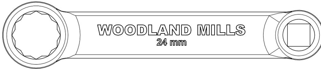
It is critical that the torque adapter be positioned 90° to the torque wrench when torquing the nuts (✓). If left straight (X), the nuts will be over-torqued and likely damage the grinder teeth threads.
