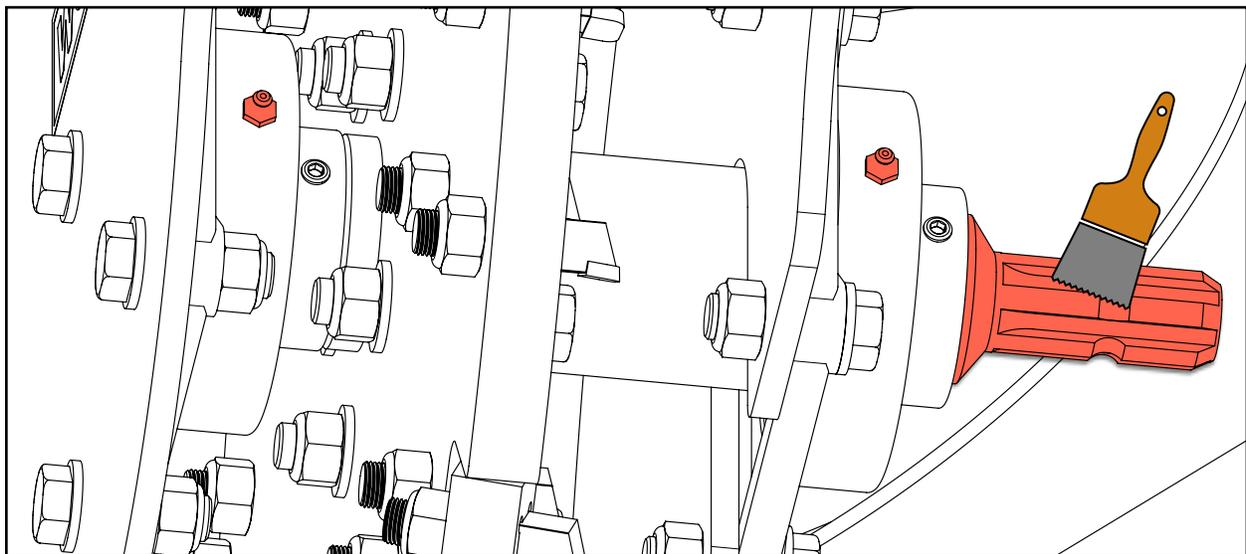
**Flywheel Shaft Bearings (Underside of Flywheel Housing) and Output Shaft**
