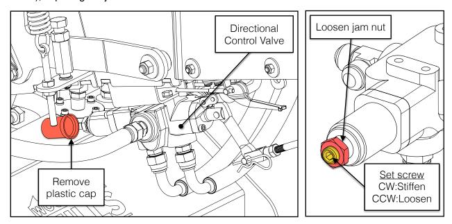
Loosen the jam nut with a 22 mm [½ in] wrench. Use a 6 mm hex key and turn the set screw *clockwise to stiffen* the movement of the arm, *counter-clockwise to loosen* it. Tighten the jam nut and replace the cap after the control arm movement feels satisfactory.
