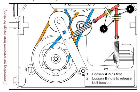
5. Unhook the extension springs from the eyebolts and allow the belt tension arms to rotate downward until they come to rest.
