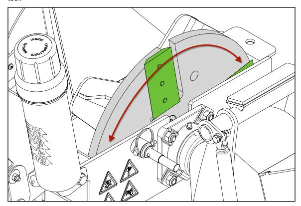
5. Place the bed plate gap tool between the bed plate and blade. Verify that the gap is consistent vertically from the top of the bed plate to the bottom.
