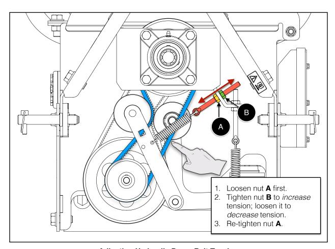
**Adjusting Hydraulic Pump Belt Tension**
