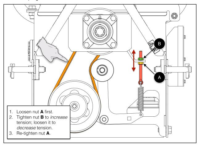
**Adjusting Secondary Flywheel Belt Tension**
