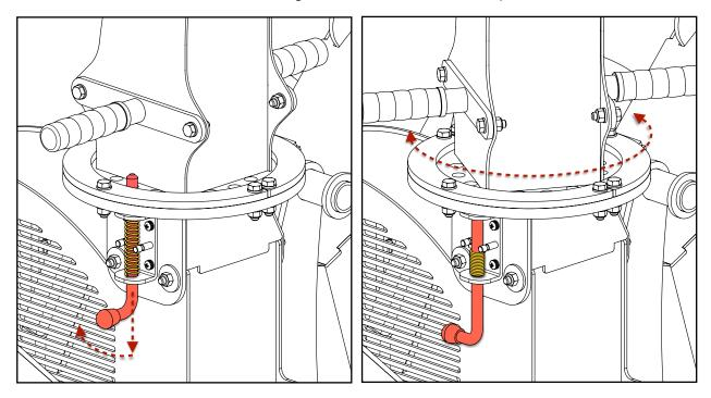
The chip deflector easily adjusts to regulate the distance the chips are thrown. Rotate the handle counterclockwise to loosen the deflector, adjust the deflector to the desired angle, then re-tighten the handle by rotating it clockwise to secure the deflector.
