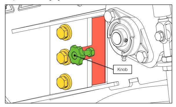
Slide the bed plate by gripping the knob and adjust its position so that it touches the bed plate gap tool. Ensure the gap is uniform along the entire edge of the blade.
