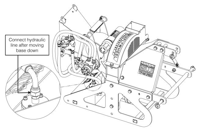
With the base secure and hydraulic line connected, slide the crate skid out from under the wood chipper and discard it.
