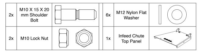
Fasten the top panel to the lower flywheel housing using two (2) M10 X 15 X 20 mm shoulder screws, six (6) M12 nylon flat washers, and two (2) M10 lock nuts to form the hinge. Tighten the hardware enough so that the hinge moves with some effort but not too tight that the nylon washers are crushed.
