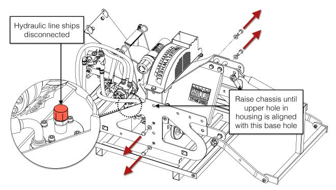
With the base separated, use the tractor's 3-point hitch to raise the chipper chassis up until the uppermost threaded holes in the side of the flywheel housing are aligned with the uppermost base holes.
