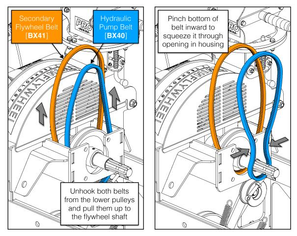
9. Reverse the steps to install new belts. Remember to install the secondary flywheel belt (rear) first before installing the hydraulic pump belt (front).
