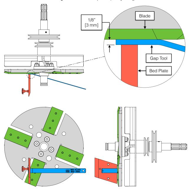
This graphic illustrates how the gap tool interfaces with the bed plate and blades in order to achieve uniform spacing. Some components removed for clarity.
