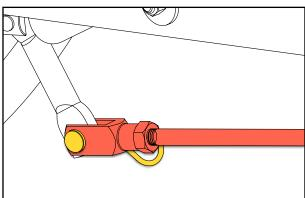
Once the linkage has been assembled, ensure both M10 jam nuts are tight.
