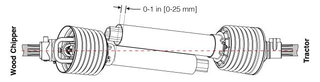
**Scenario 3.** If the guard tube end extends past the shroud collar, hold a straight edge firmly against the shroud collar so that it lays across the outer guard. Mark the position on the outer guard.
