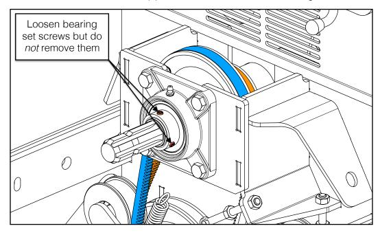
7. Remove the four (4) M12 X 40 mm hex bolts and lock nuts used to mount the bearing and slide it off the flywheel shaft. The shaft may tilt downward once the bolts are removed but this normal.
