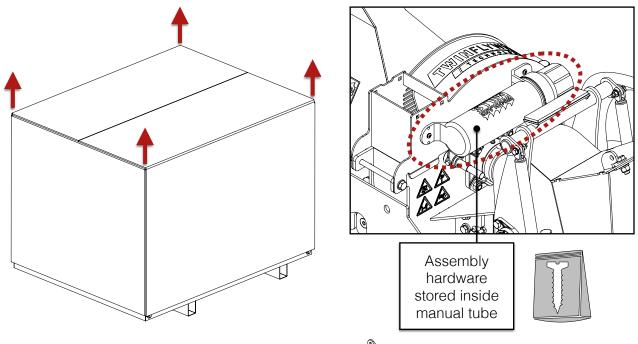
Remove all the loose components from the skid (infeed chute panels, control arm, edge bar, control arm linkage, discharge chute, discharge chute handles, PTO shaft) and set them to the side. Leave the wood chipper on the skid.
