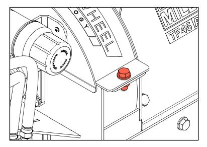
3. With the primary flywheel exposed, manually rotate it so that one of the four (4) locking holes in the flywheel (near the front of the blade) approximately lines up with the flywheel lock pin at the rear of the housing. Remove the small locking pin from the flywheel lock pin and flip the flywheel lock pin around 180°, passing it through the housing and into the locking hole in the primary flywheel. Reinstall the smaller locking pin to the flywheel lock pin.
