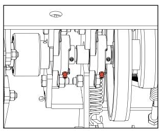
**Pump Shaft Bearings (2x Underside)**
