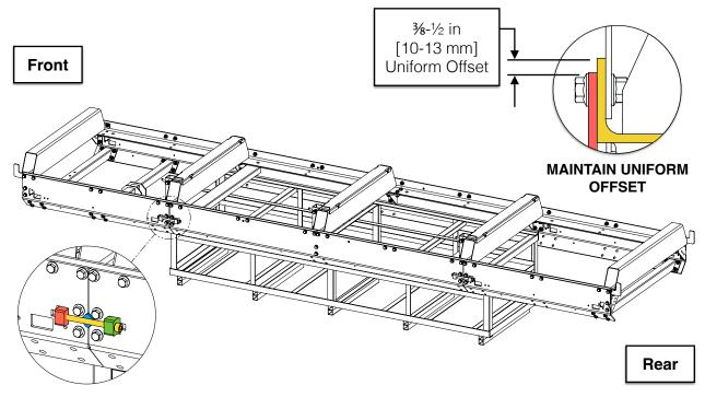
While maintaining a uniform side plate-to-rail offset, torque the remaining bolts per the table in section, *BOLT TORQUE SPECIFICATIONS*, starting from the centre and working towards the outer ends. Torque the M10x120 socket head cap screws used for the side plate alignment. Ensure the track is straight, level, and square during this procedure.
