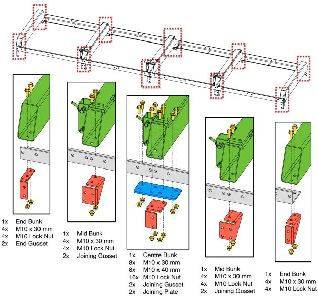
The above steps need to be completed on both left and right sides of the track. Make sure the gussets are flush with the outside face of the track rails as shown below.
