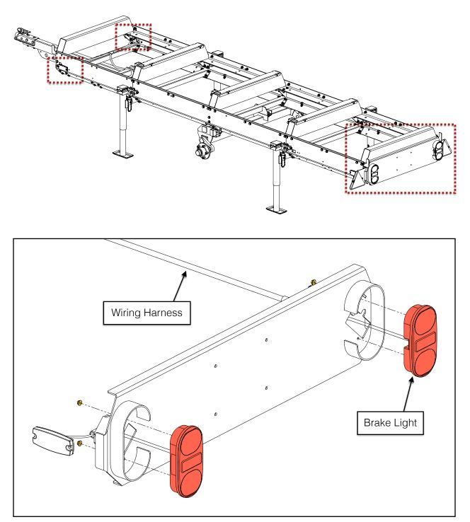
\*\*Note: Tail lights (North America and Europe) and side lights (North America only) are integral to the wire harness. They are shown exploded for assembly clarity.\*\*
