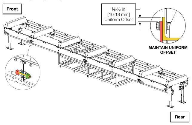
While maintaining a uniform side plate-to-rail offset, torque the remaining bolts per the table in section, *BOLT TORQUE SPECIFICATIONS*, starting from the centre and working towards the outer ends. Torque the six (6) M10x120 socket head cap screws installed in all prior steps. Ensure the track is straight, level, and square during this procedure.
