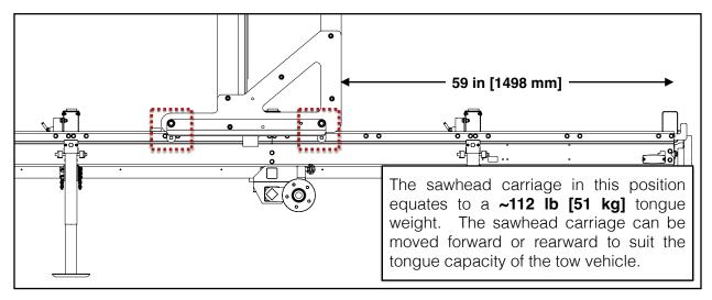
\*\*Note: Tolerance on tongue weights is approx. ±15 lb [±7 kg] depending on how many accessories are installed (Lap Siding, Power Head, Log Loading Ramp Kit, Toolbox, Cant Hook, etc.)\*\*
