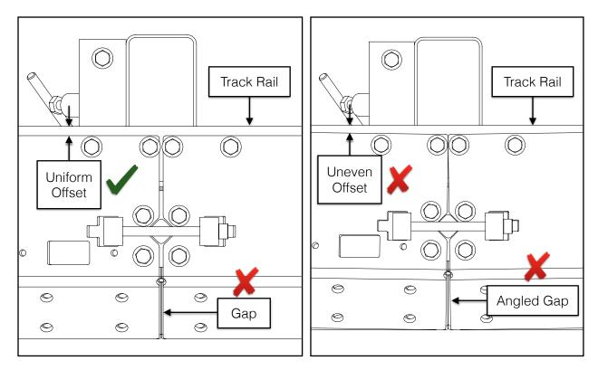
If there are gaps, they can be closed by tightening the M10 X 120 mm Socket Head Cap Screws.
