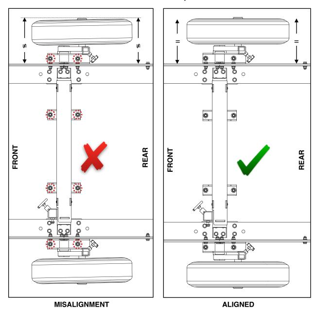
If the wheels are parallel, tighten the axle bolts to the **specified torque** and proceed to the next section. However, if the wheels are *not* parallel, loosen the four (4) M12 bolts on the affected axle(s). Rotate the axle assembly and wheel until the wheels are parallel. Then tighten the axle bolts to the **specified torque**.
