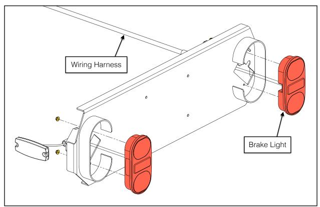
\*\*Note: Tail lights (North America and Europe) and side lights (North America only) are integral to the wire harness. They are shown exploded for assembly clarity.\*\*
