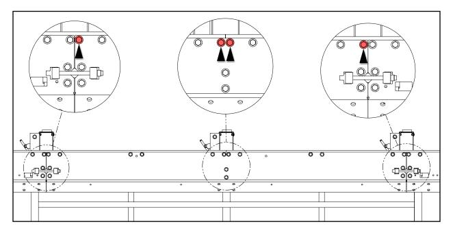
With the long side plate secured in place, note the gaps (if any) between the short side plates and the long side plates.
