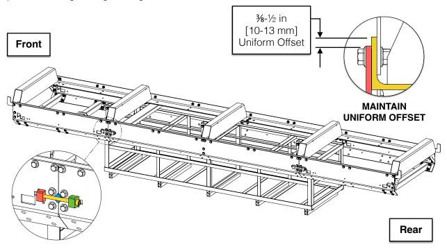
While maintaining a uniform side plate-to-rail offset, torque the remaining bolts per the table in section, *BOLT TORQUE SPECIFICATIONS*, starting from the centre and working towards the outer ends. Torque the M10x120 socket head cap screws used for the side plate alignment. Ensure the track is straight, level, and square during this procedure.
