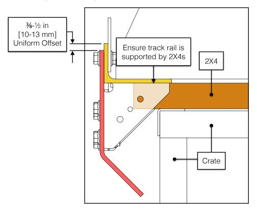
If the offset is not uniform, ensure the track is sitting on the 2X4s and not the crate. The side plates need to hang from the rails unobstructed, with only the force of gravity pulling them down.
