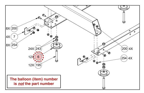
Next, turn to the *Parts Lists* section and locate the balloon number in the "Item" column:
