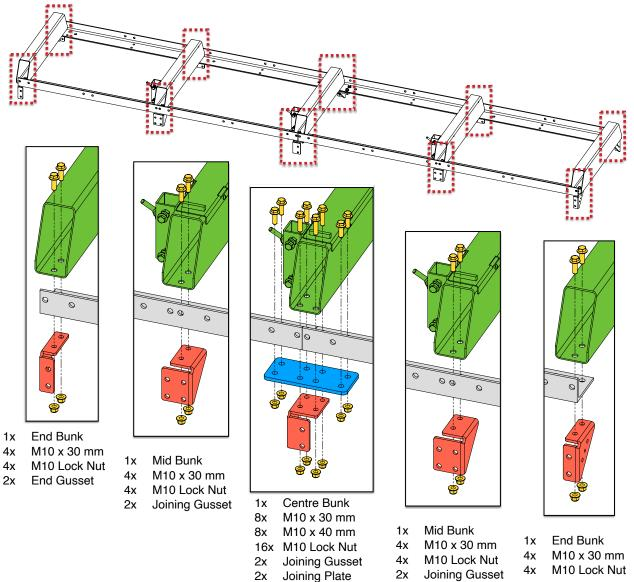
The above steps need to be completed on both left and right sides of the track. Make sure the gussets are flush with the outside face of the track rails as shown below.
