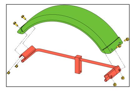
Slide the post on the fender bracket into the sleeve on the axle mount and insert the locking pin through the hole located at the bottom of the fender bracket post. Secure the fender/fender bracket sub-assembly using the M10 X 30 mm knob by threading it into the axle mount until tight.
