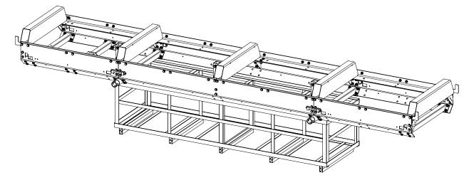
Slide the swivel jacks onto the jack mounts and secure them with the locking pins. Raise the jacks up to slide the crate out from under the trailer assembly. Place blocks of wood underneath each jack if necessary to achieve the required clearance.
