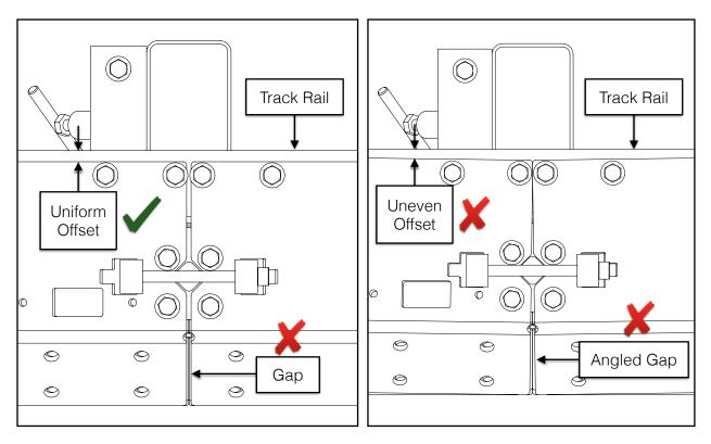
If there are gaps, they can be closed by tightening the M10 X 120 mm Socket Head Cap Screw.
