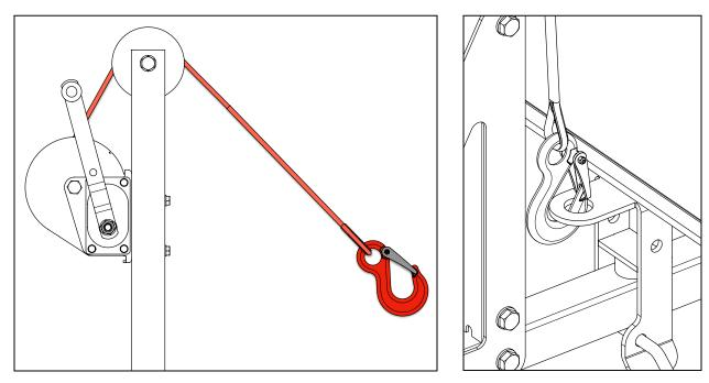
Use the winch to wind any slack out of the winch rope so that the hook does not rattle around during travel.
