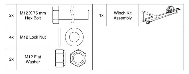
Assemble the winch kit to the chassis draw bar using two (2) M12 X 75 mm hex bolts, four (4) M12 flat washers, and two (2) M12 lock nuts. Fully tighten *all* the hardware.
