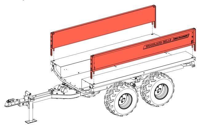
On both ends of each side panel, secure the panel to the bed. Thread one (1) M10 X 25 mm hex head bolt, one (1) M10 fender washer, and one (1) spacer through the side panel hinge slot and into the threaded hole in the hinge block as shown below. Tighten all the hardware.
