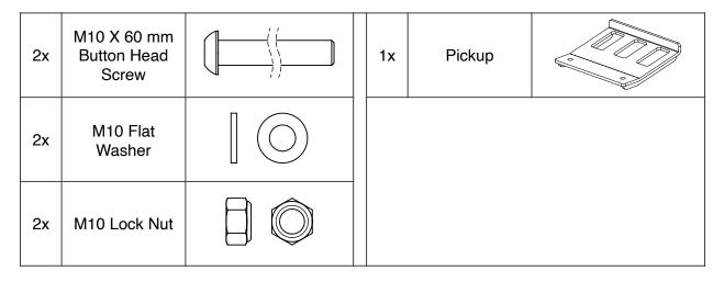
Use two (2) M10 X 60 mm button head screws, two (2) M10 flat washers, and two (2) M10 lock nuts to secure the pickup to the front support rib.
