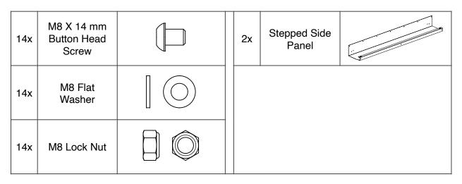
Use seven (7) M8 X 14 mm button head screws, seven (7) M8 flat washers, and seven (7) M8 lock nuts to join each stepped side panel to the bed panel. Do *not* fully tighten any of the hardware until instructed.
