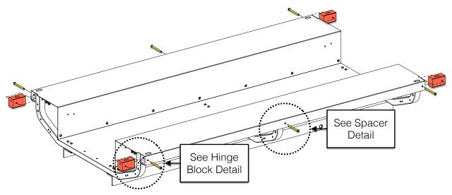
At the midpoint of each side panel, use one (1) M8 X 100 mm button head screw, one (1) M8 flat washer, and one (1) M8 lock nut to join the panel to the centre support rib using the 8 X 12 X 48 mm spacer.
