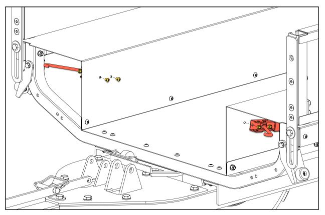
Before installing the tailgate assembly on the utility box, verify that the four (4) button head screws along the top the tailgate assembly are fully tightened before installation.
