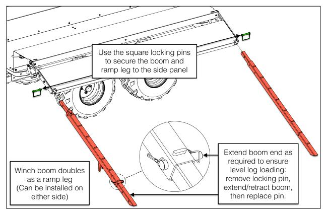
7. INSERT THE BOOM AND RAMP LEG INTO THE OPENINGS AT THE TOP OF EACH END OF THE SIDE PANEL AND SECURE THEM WITH THE SQUARE LOCKING PINS.
