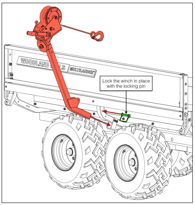
8. SLIDE THE WINCH POST ASSEMBLY INTO THE WINCH BRACKET BETWEEN THE TWO WHEELS AND LOCK IT IN PLACE WITH THE SQUARE LOCKING PIN.
