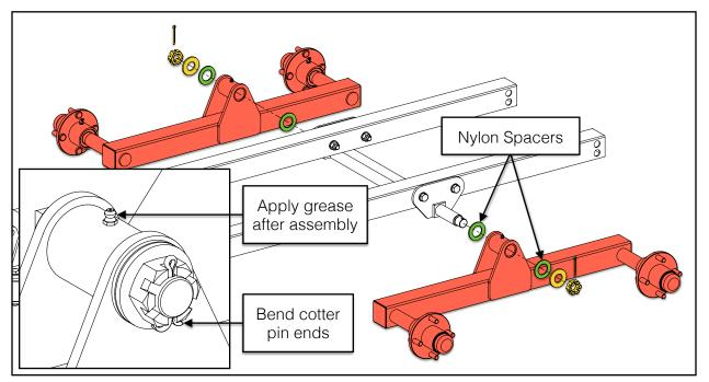
\*\*Note: Add grease to walking beam pivots after assembly.\*\*
