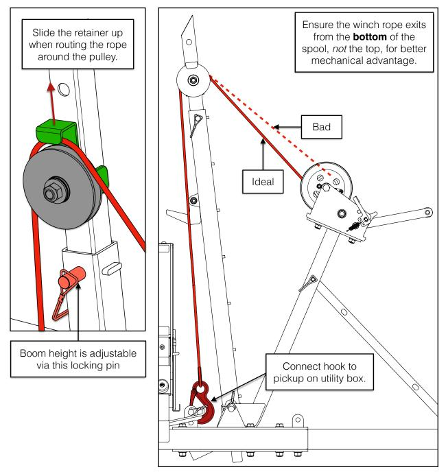
Note: If the winch shipped with the rope exiting the top of the spool, it will need to be unwound and then rewound in the opposite direction.
