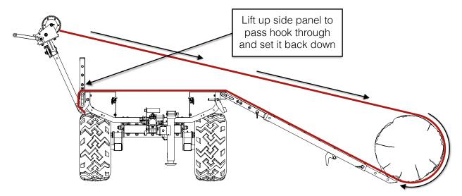
The rope must route over and around the log and back up *under* the vertical side panel (lift the side panel up high enough to pass the hook through and set it back down on the rope). Secure the hook to the inside of the end of the winch post around the winch bracket as shown.
