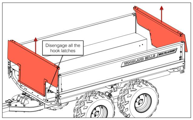
5. DISENGAGE ALL THE HOOK LATCHES AND REMOVE BOTH TAILGATES.
