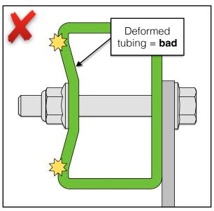
DO <u>NOT</u> TORQUE TO SPEC WHEN BOLTING THROUGH TUBING. SNUG HARDWARE, THEN TIGHTEN A FURTHER <sup>1</sup>/<sub>4</sub>-<sup>1</sup>/<sub>2</sub> TURN.
