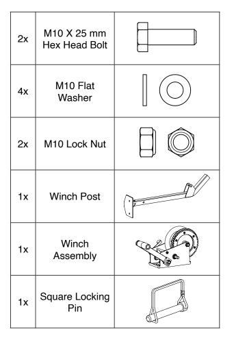
Use two (2) M10 X 25 mm hex bolts, four (4) M10 flat washers, and two (2) M10 lock nuts to join the winch to the winch post.
