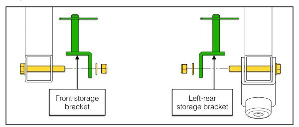
To mount the front storage bracket to the *middle* support rib, use one (1) M8 X 60 mm hex head bolt, two (2) M8 flat washers, and one (1) M8 lock nut.
