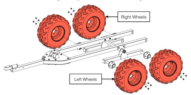
The tires are shipped without air. Inflate the tires to the manufacturer's recommended pressure located on the tire sidewall.
