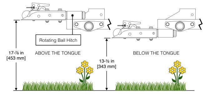
With the *Below the Tongue* style, the tongue is flipped 180° so that the rotating ball hitch is on the bottom.
