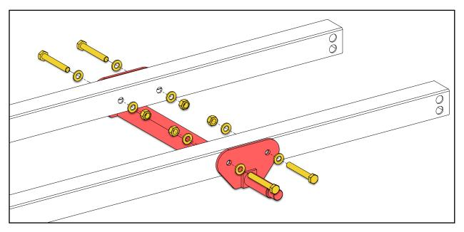
Check the chassis for squareness by measuring diagonally from the end of each rail to the back edge of the top tongue plate. Once square, tighten all the hardware from this and the previous step.
