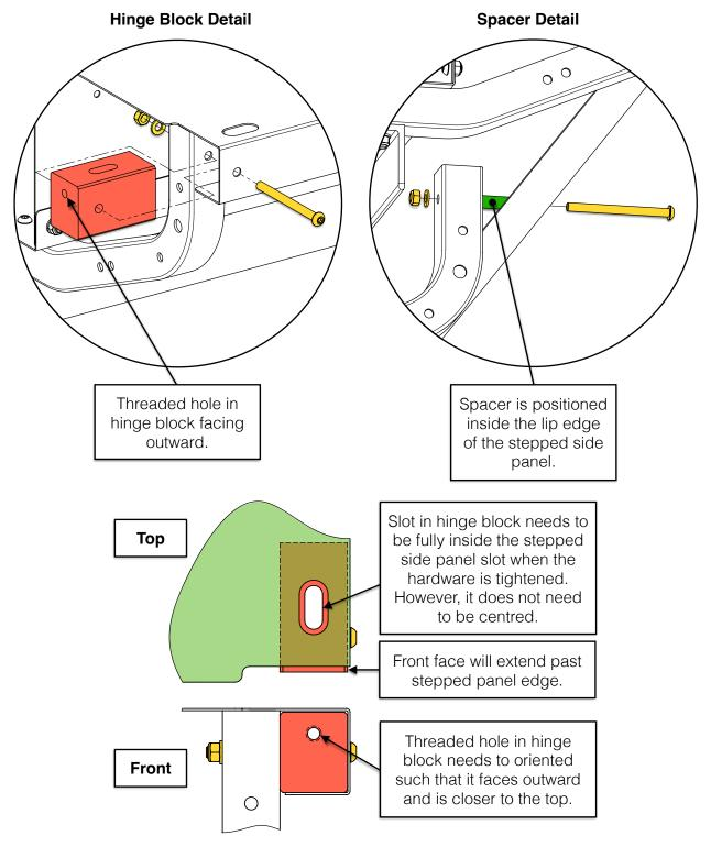
Do not fully tighten any of the hardware until instructed.
