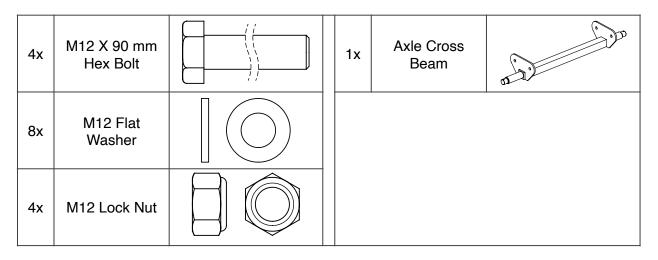
Use four (4) M12 X 90 mm hex bolts, eight (8) M12 flat washers, and four (4) M12 lock nuts to join the axle cross beam to the side rails.
