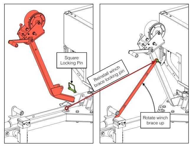
Disconnect the square locking pin from the winch brace, rotate the brace up, and reinstall the square locking pin through the hole in the end of the brace and the hole near the top of the winch post.
