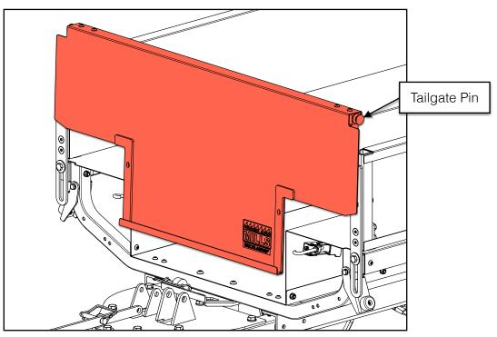
Then secure the tailgates to the utility box with the hook latches. Adjust the engagement of the hook latches using the jam nut on the latch.
